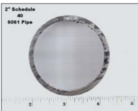
2" schedule 40 aluminum pipe frame 2.375" O.D. – 2.067" I.D.
